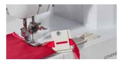
**Bias tape binding set** For folding and attaching 6mm or 12mm-wide bias tapes to fabric edge.
